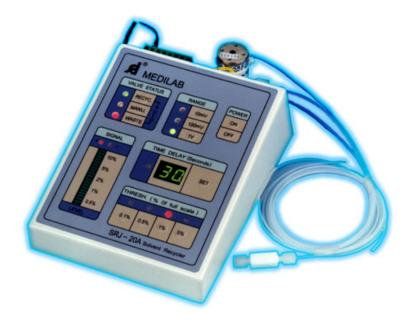
Intelligent mobile phase recycling is accomplished by placing an electrically actuated Recycle Valve in the fluid path between the HPLC detector and the solvent waste reservoir. The signal processor in the Recycler SRJ-20A, which monitors the detector signal to determine when peaks and other contaminants are passing through the detector flow cell, controls the valve.
